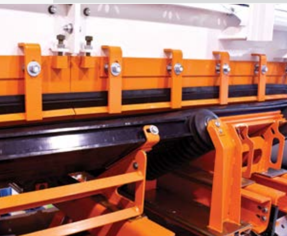
Components are designed to contain fast-moving loads to control spillage and minimize dust.
